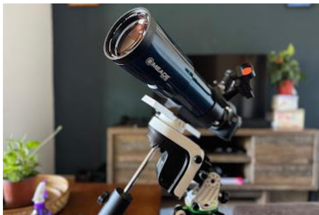
My telescope configuration – a Meade 80mm refractor telescope and Canon DSLR on top of a SkyWatcher Az-GTI tracking mount, controlled by a smartphone app or via laptop
